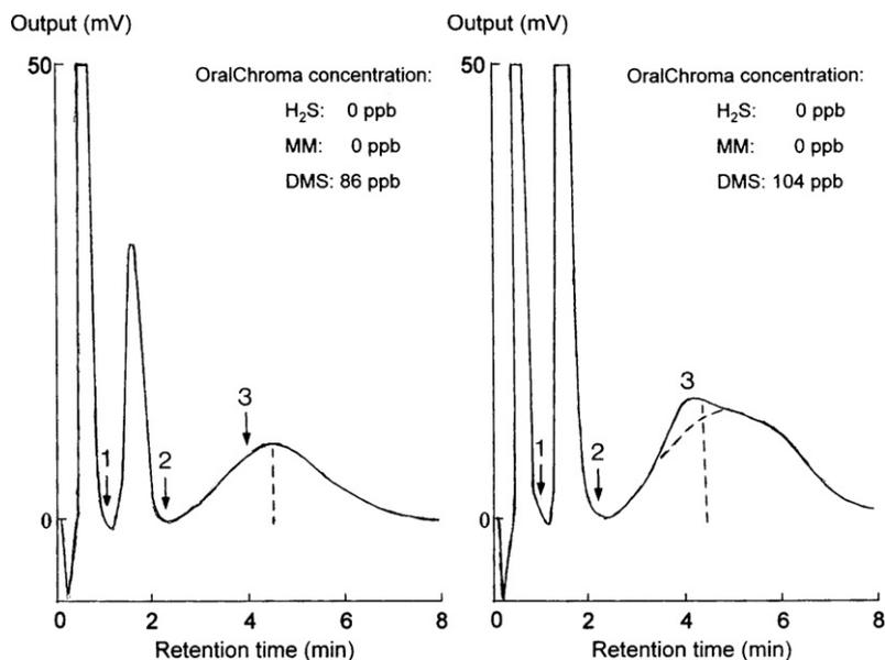
**Figure 5.** Disturbance by a broad peak, originated from the rubber barrel seal of the used syringe, in the OralChroma chromatogram of the breath of a normal person (left panel) and of the breath of a patient with extra-oral halitosis (right panel). Peak assignment: 1 = H<sub>2</sub>S, 2 = MM, 3 = DMS.
