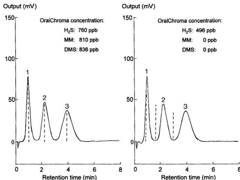
**Figure 4.** OralChroma chromatograms of a standard mixture of 1000 ppb each of H<sub>2</sub>S, MM and DMS. Injection: 0.5 ml. The vertical dotted lines represent the assignment by OralChroma of H<sub>2</sub>S, MM and DMS, respectively. Left panel: correct assignment by OralChroma. Right panel: incorrect assignment by OralChroma. Peak assignment: 1 = H<sub>2</sub>S, 2 = MM, 3 = DMS.
