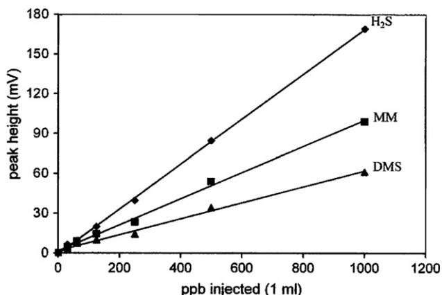
**Figure 6.** Standard calibration graphs of H<sub>2</sub>S, MM and DMS. Plot of concentration injected (1 ml) against the peak height (mV).
